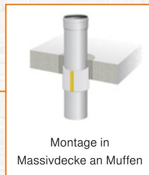
Montage in Massivdecke an Muffen
